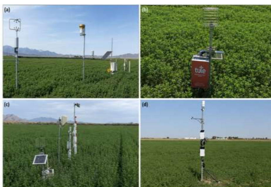
Figure 12. Precision irrigation monitoring technologies deployed in commercial forage production systems in California's low desert, including (a) eddy covariance evapotranspiration (ET) tower, (b) Tule evapotranspiration sensor, (c) automated weather and telemetry station, and (d) wireless soil moisture and environmental monitoring node. These integrated monitoring systems support evapotranspiration-based irrigation scheduling, root-zone storage management, drought adaptation, and real-time decision support frameworks.
